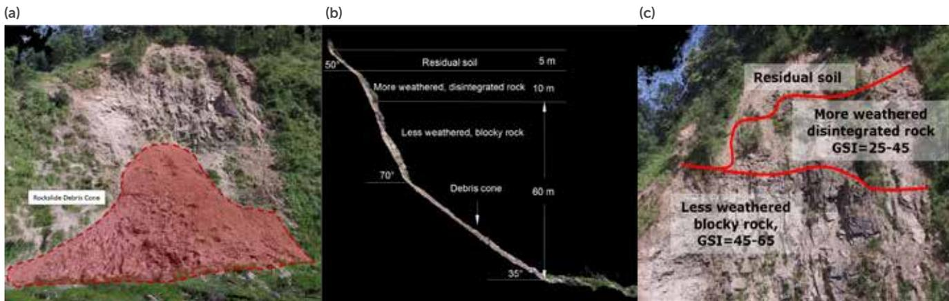
**Figure 5.** Characterization of a 75-m-high co-seismic rock slide in Nepal during the 2015 Gorkha earthquake. (a) 3D rock mass characterization; (b) cross-section through slide; (c) geomechanical characterization of rock mass.
