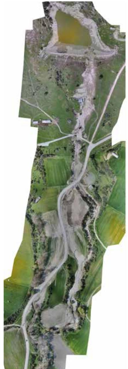
**Figure 4.** Orthophoto of original water impoundment area, failed dam, and flooded area downstream of the failure location. The water travelled about 1 km downstream before reaching a natural gully and stream.
