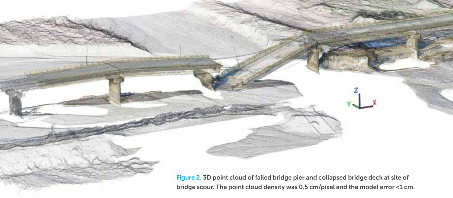
**Figure 2.** 3D point cloud of failed bridge pier and collapsed bridge deck at site of bridge scour. The point cloud density was 0.5 cm/pixel and the model error <1 cm.
